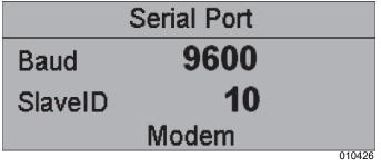
Figure 2-15. Serial Port Page. If modem is not connected, RS232 displays in place of Modem.
