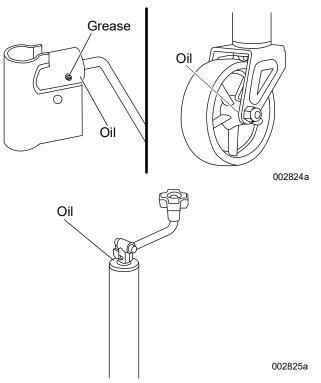
Figure 4-3. Lubrication Points
