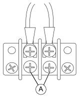
Figure 3-1. Remote Start Terminal Block
