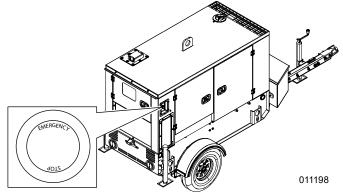
Figure 3-10. Emergency Stop Switch
