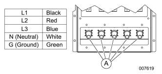
Figure 3-5. Cam Lock Connections
