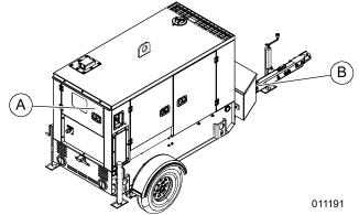
Figure 2-2. Unit and Serial Number Locations
