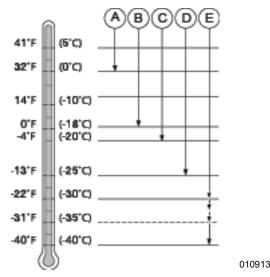
Figure 3-2. Cold Weather Starting Guidelines
