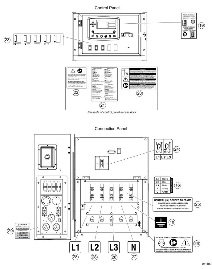
Figure 1-3. Control Panel and Connection Panel Decals
