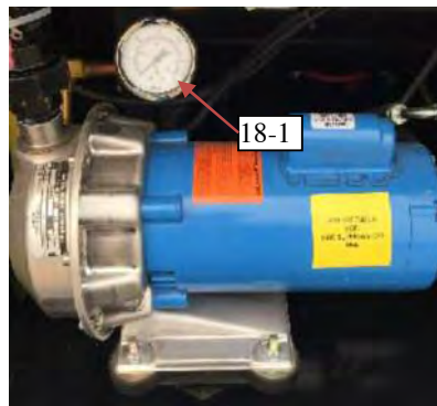
18-system pressure gauge
