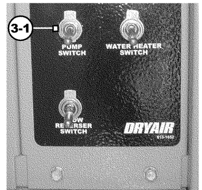
3 - pump, water heater & flow reverser switch
