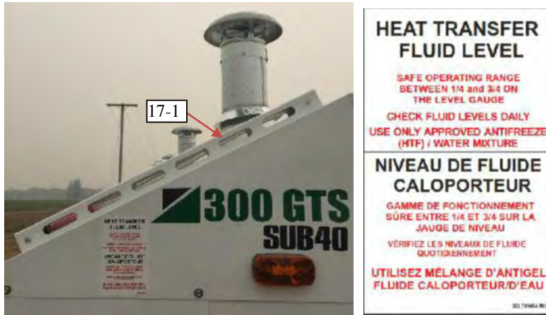
17-heat transfer fluid sight glass
