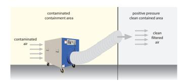
To create **POSITIVE PRESSURE** inside the containment, more air has to be pumped in than leaks out of the containment. Place the machine outside the containment and hook a flexible duct to the outlet ring of the machine ducting the exhaust into the containment. (See Above)
