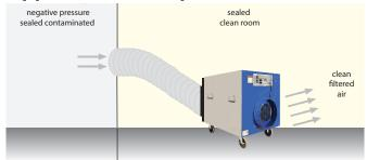
To create **NEGATIVE PRESSURE** inside the containment, more air has to be exhausted out than leaks into the containment. Place the machine inside the containment and hook a flexible duct to the outlet ring of the machine exhausting to outside the containment. (See Above) All of the air being exhausted has been treated by the HEPA filter so no contaminants are being exhausted from the containment.
