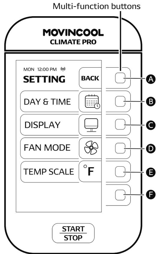
4. Press **C** or **E** to adjust the brightness level and then press **D** to save.
