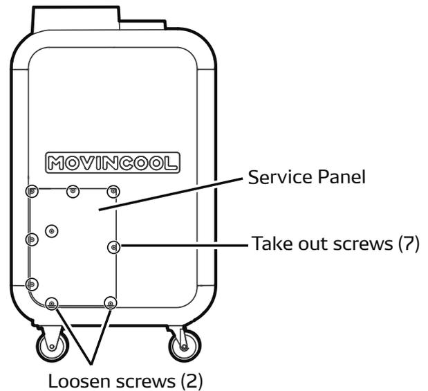
3. Loosen the center bottom screw and take out the other seven (7) screws. Move the upper rear panel upward and remove it.
