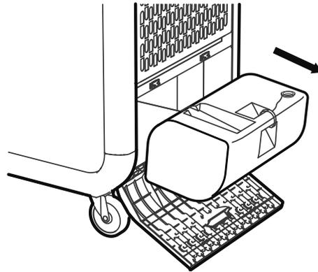
3. Remove the cap and empty the tank.
