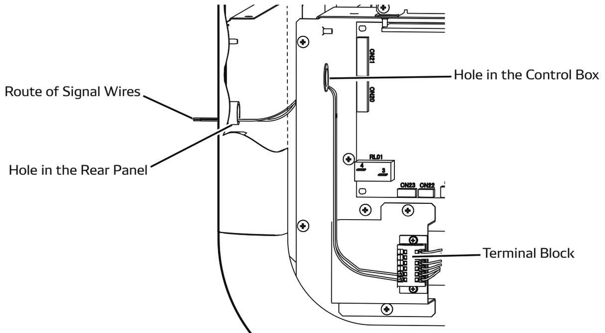
6. Connect the warning signal wires to the terminals OS-1 and OS-2 as shown in the figure.
