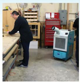
**Cooling:** Self-contained, portable MovinCool units provide quick, cooling relief for personnel in job-site trailers or tents — or for building occupants when the central HVAC system is temporarily turned off.
